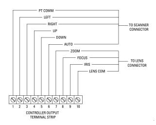
Figure 2. MPTAZ24DT, MPTAZ24DT/220 Wiring Diagram for Scanners and Lenses
